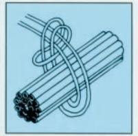
Western Filament lacing tapes are flat bra yarns in accordance with MIL-T-43435, and m
