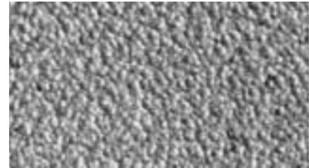
Magnification of peened surface.
