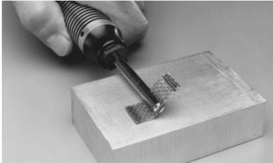
Peen surface with a circular motion. Tool must be pre-set to a constant torque.
