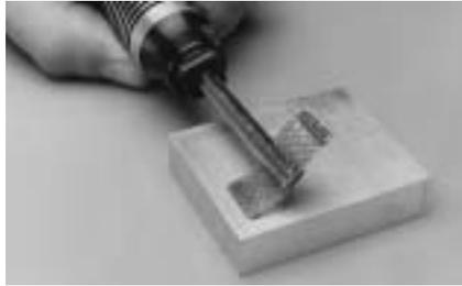
**Flat surface** 2" x 2 1/4" peened to 12 Almen "A" intensity with a 9/16" x 1 1/4" flap.
