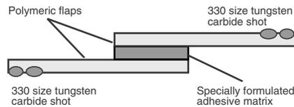
The flap/mandrel assemblies provide convenient portability and are especially effective for precision in-service rework, manufacturing, repair of small areas, and peening holes with diameters down to 1/2" (12.7mm).
