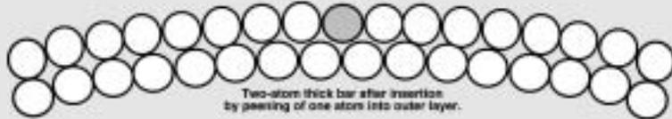
Two-atom thick bar after insertion by peening of one atom into outer layer.
