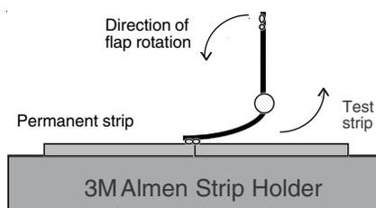
**NOTE:** Generally you will peen the surface with the flap rotating away from the permanent strip (as shown below left).
